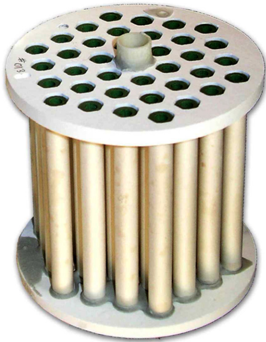
Fig. 1. Photograph of a tubular SOFC stack consisting of three hexagonal rings.
